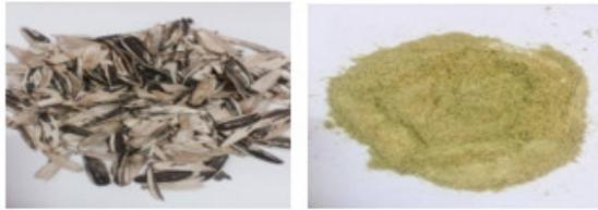
**Figure 1:** Sunflower wastes before and after grinding
