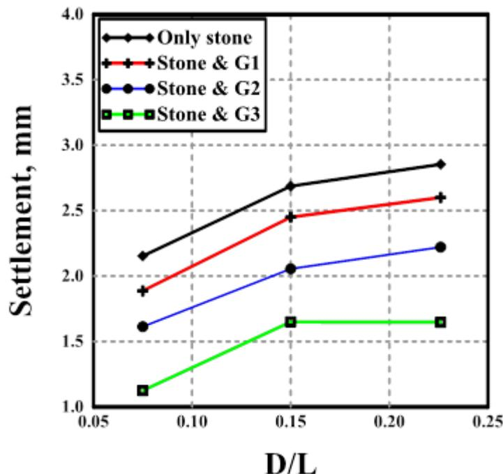
Fig. 4: D/L ratio with settlement for a sample having a diameter 3 cm under a load of 50 kN.
