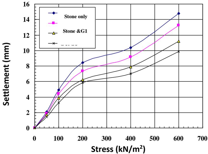
Fig. 23: Stress-settlement for sample having a diameter of 5 cm and  $D/L=0.25$ .
