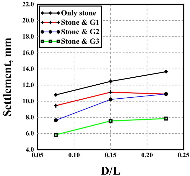
Fig. 7: D/L ratio with settlement for a sample having a diameter 3 cm under a load of 400 kN.
