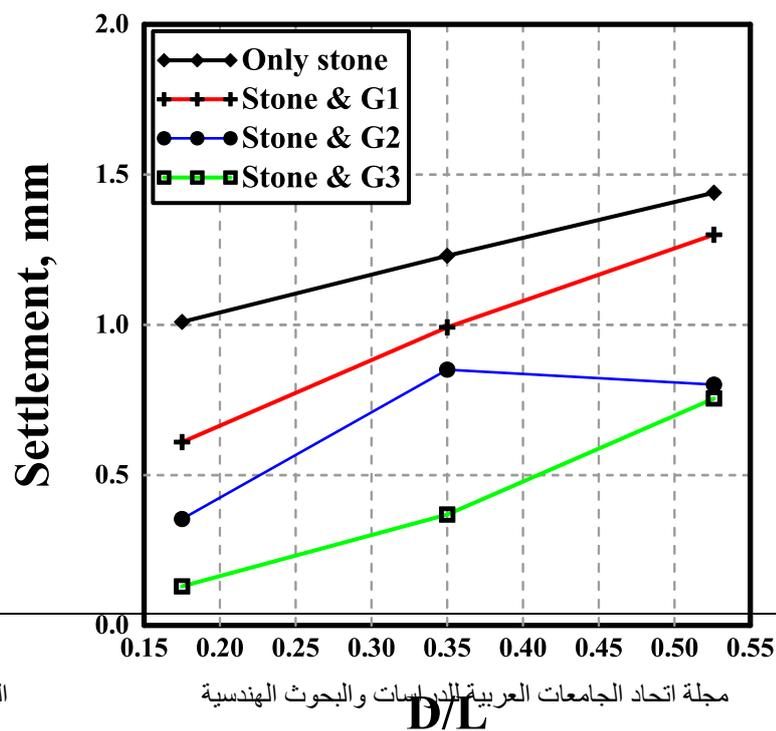
Fig. 14: D/L ratio with settlement for a sample having a diameter 7 cm under a load 50 kN.
