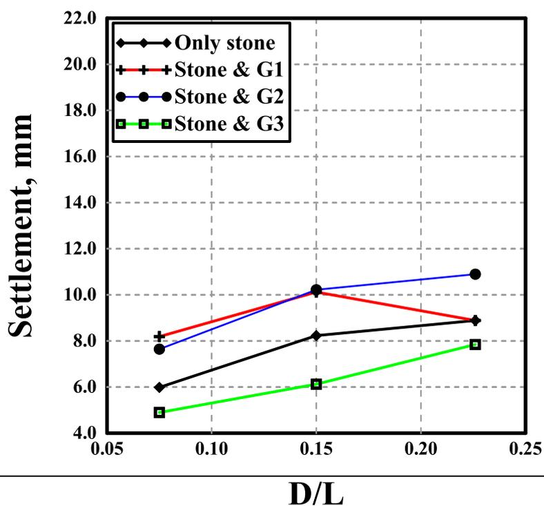
Fig. 6: D/L ratio with settlement for a sample having a diameter 3 cm under a load of 200 kN.
