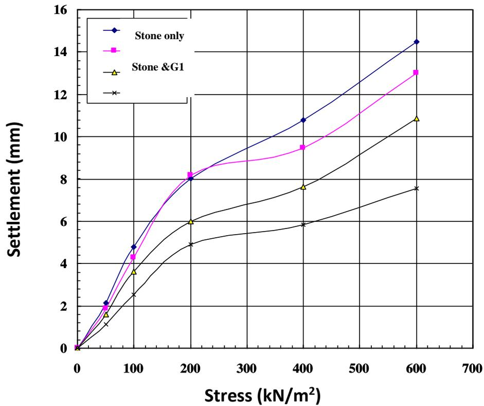
Fig. 19: Stress-settlement for sample having a diameter of 3 cm and D/L=0.075.
