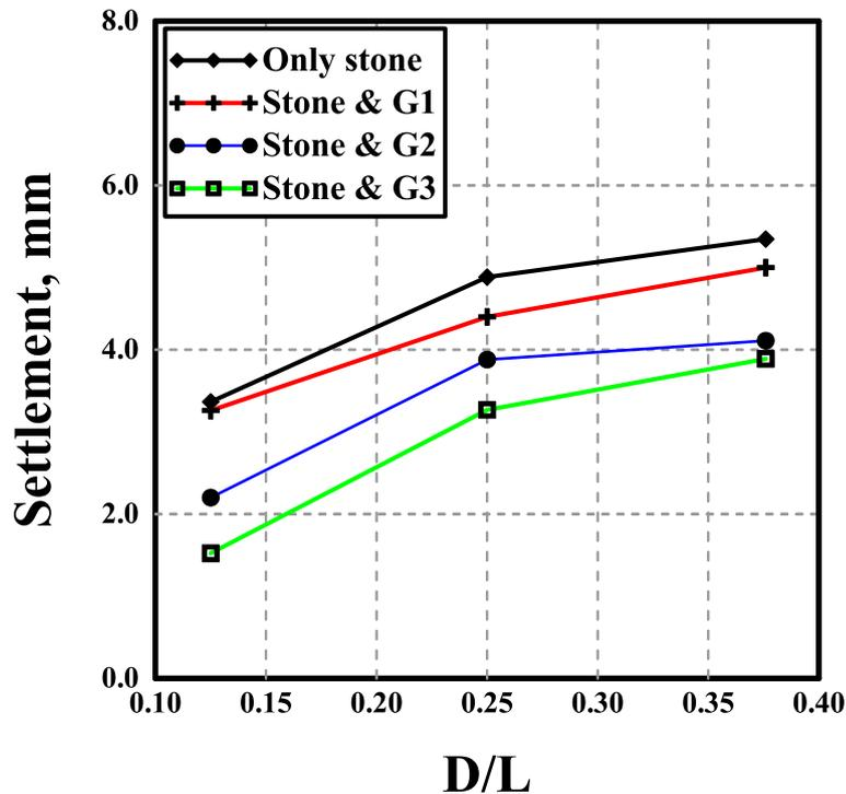
Fig. 10: D/L ratio with settlement for a sample having a diameter 5 cm under a load of 100 kN.
