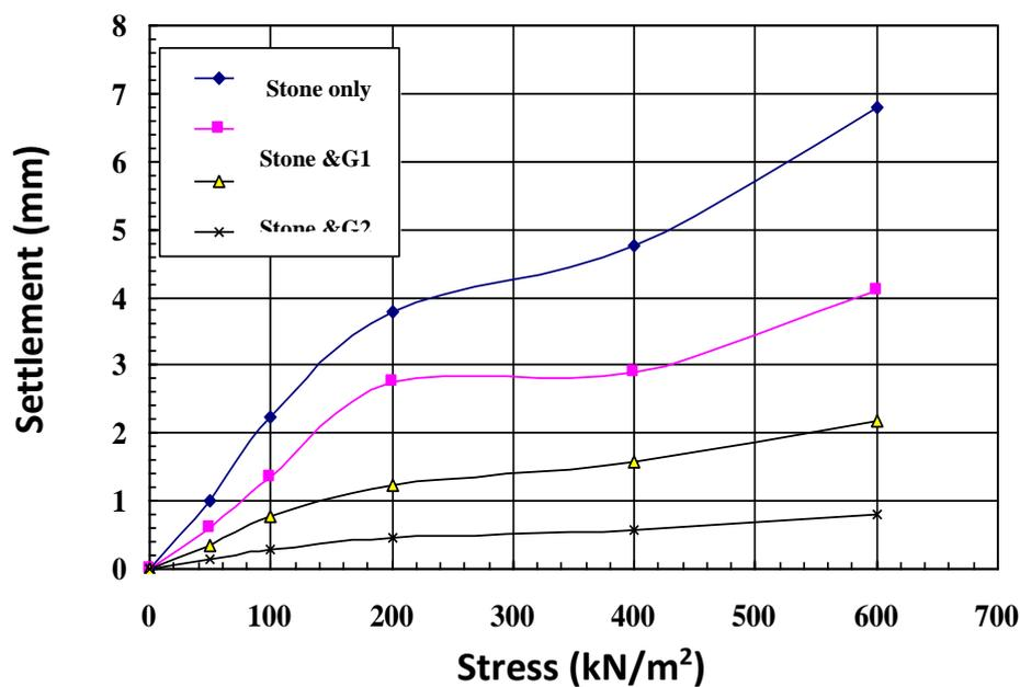
Fig. 25: Stress-settlement for sample having a diameter of 7 cm and  $D/L=0.175$ .
