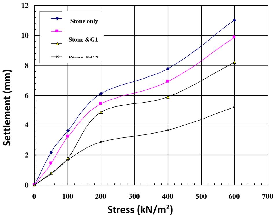
Fig. 21: Stress-settlement for sample having a diameter of 3 cm and D/L=0.526.
