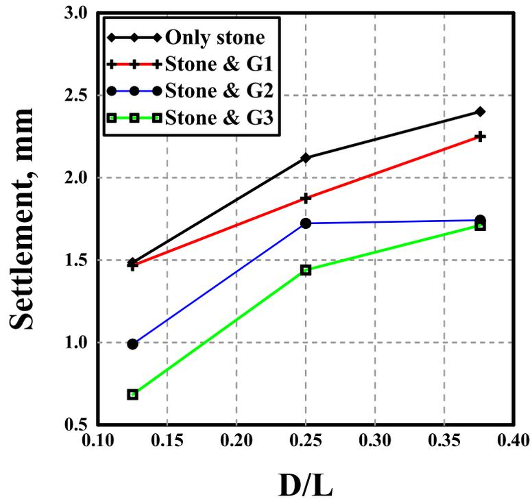
Fig. 9: D/L ratio with settlement for a sample having a diameter 5 cm under a load of 50 kN.
