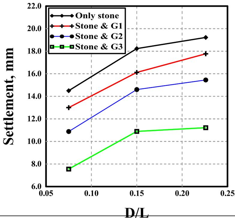
Fig. 8: D/L ratio with settlement for a sample having a diameter 3 cm under a load of 600 kN.
