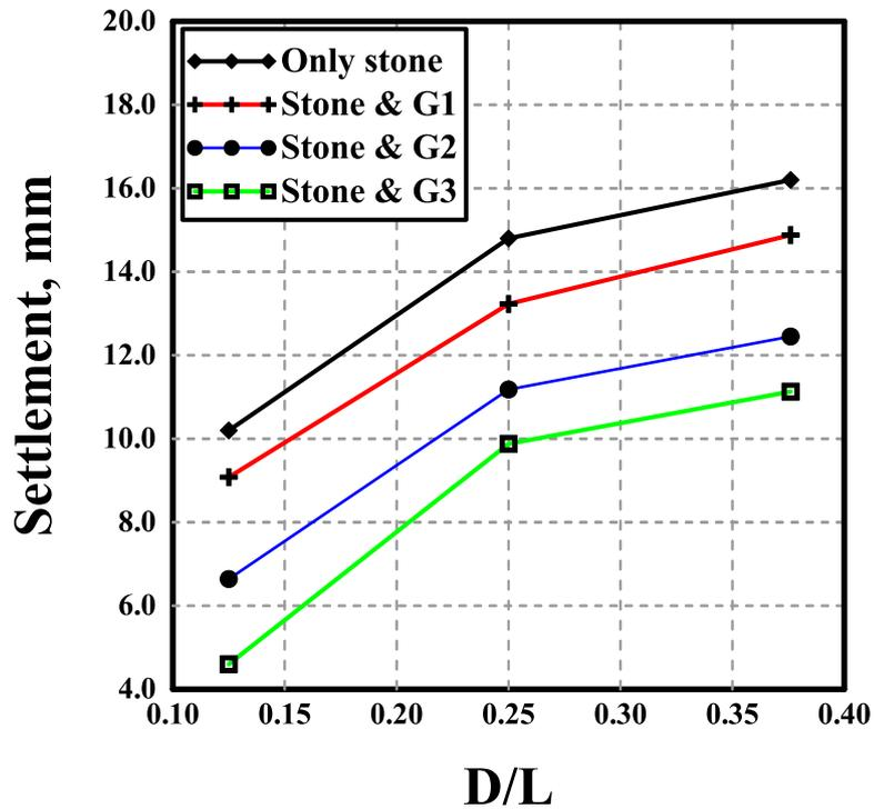
Fig. 13: D/L ratio with settlement for a sample having a diameter 5 cm under a load 600 kN.
