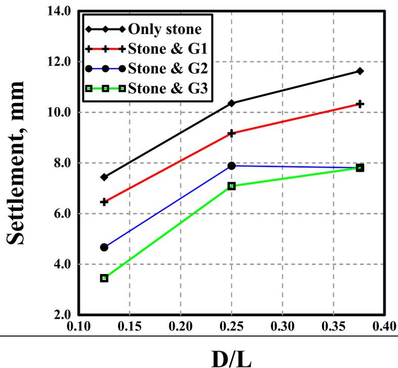
Fig. 12: D/L ratio with settlement for a sample having a diameter 5 cm under a load 400 kN.
