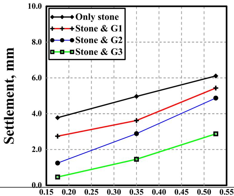
Fig. 16: D/L ratio with settlement for a sample having a diameter 7 cm under a load 200 kN.
