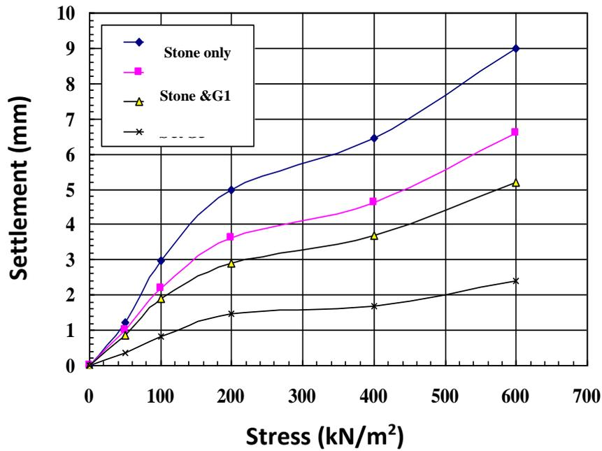
Fig. 26: Stress-settlement for sample having a diameter of 7 cm and D/L=0.35.
