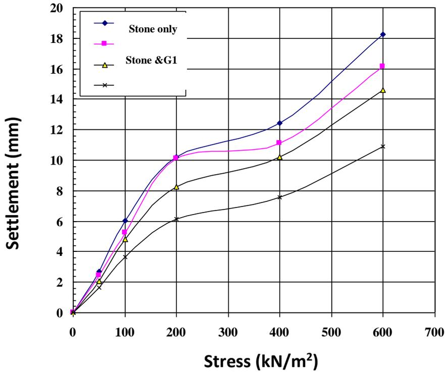
Fig. 20: Stress-settlement for sample having a diameter of 3 cm and D/L=0.15.
