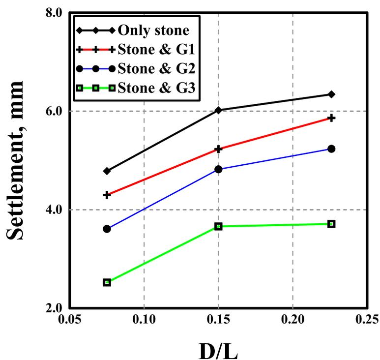
Fig. 5: D/L ratio with settlement for a sample having a diameter 3 cm under a load of 100 kN.
