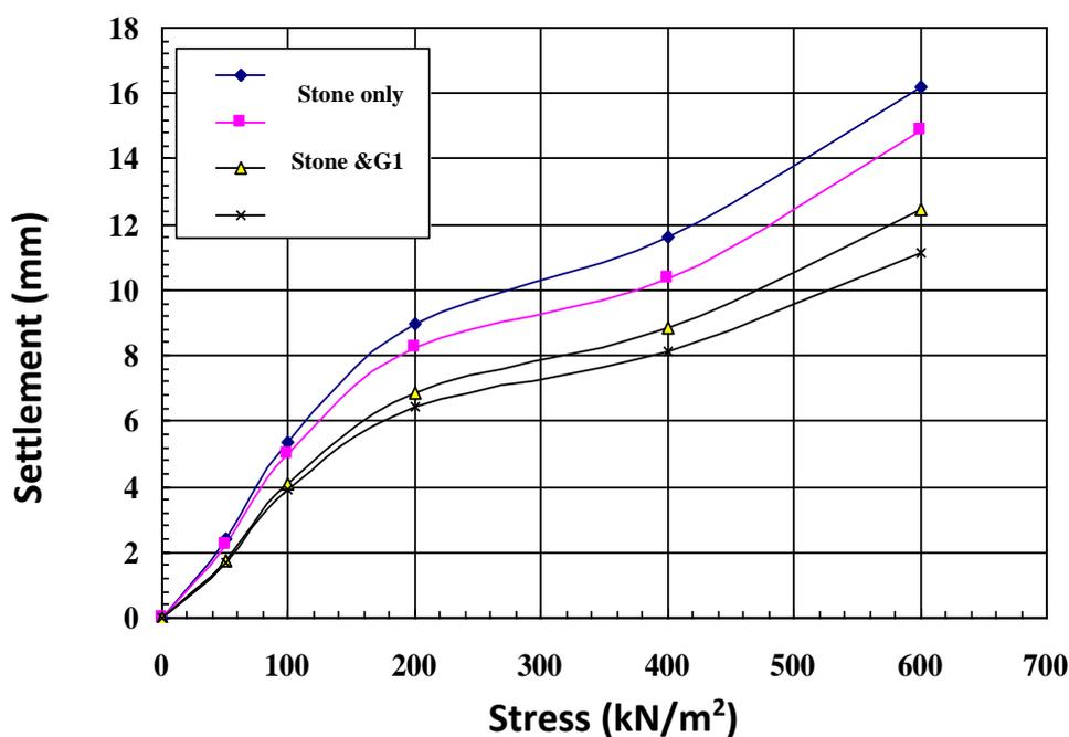
Fig. 24: Stress-settlement for sample having a diameter of 5 cm and  $D/L=0.376$ .
