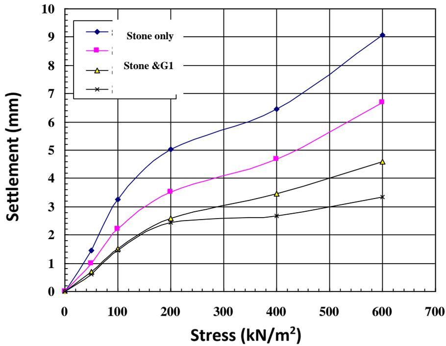
Fig. 22: Stress-settlement for sample having a diameter of 5 cm and  $D/L=0.125$ .
