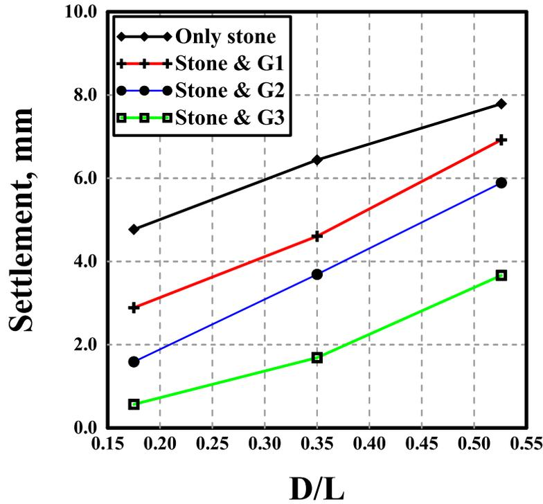
Fig. 17: D/L ratio with settlement for a sample having a diameter 7 cm under a load 400 kN.
