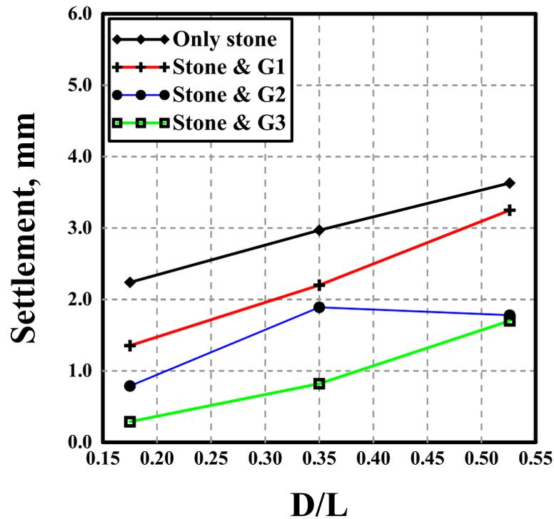
Fig. 15: D/L ratio with settlement for a sample having a diameter 7 cm under a load 100 kN.
