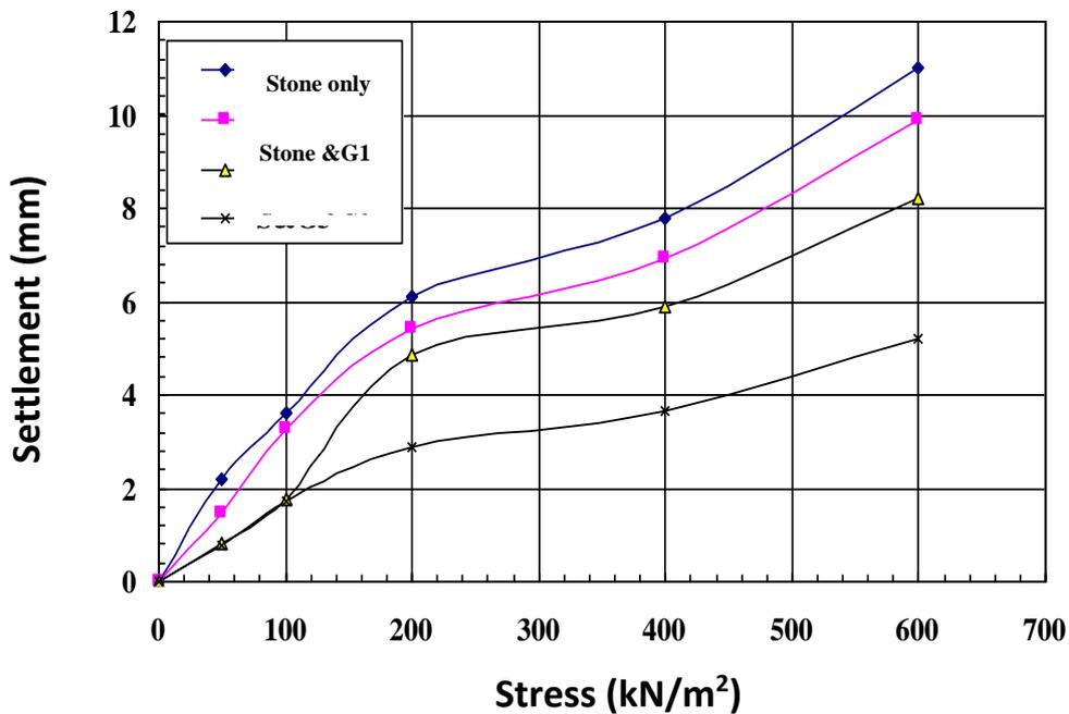
Fig. 27: Stress-settlement for sample having a diameter of 7 cm and D/L=0.526.
