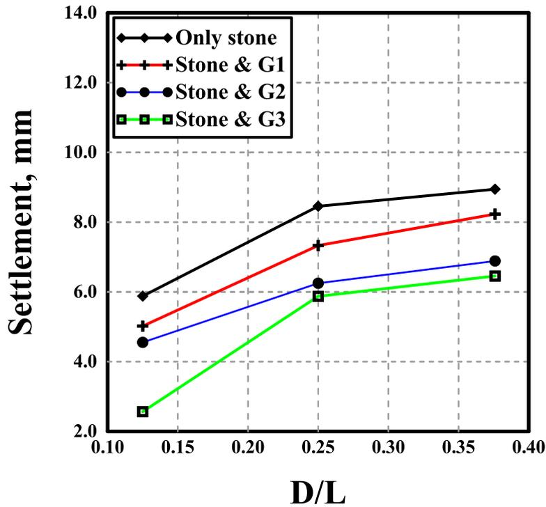
Fig. 11: D/L ratio with settlement for a sample having a diameter 5cm under a load of 200 kN.
