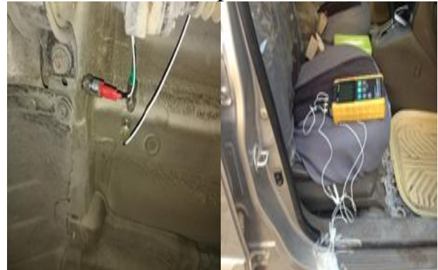
Fig.7 Vibration meter and sensors used to investigate road vehicle vibrations
